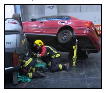
considered. This is where crew members support the vehicle, restricting its movement, whilst a medic gains access to perform a lifesaving intervention. For example, when a car is on all four wheels, crew members can brace the vehicle by the wheel This stops the vehicle dropping on its suspension when the medic enters the vehicle and
