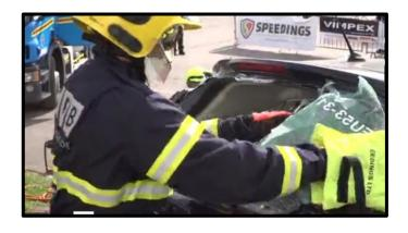
Since 1980, when it became legislation in the UK for front screens to be made of specified safety glass, generally vehicles have been fitted with a laminated front screen and toughened glass down the sides and at the rear.
