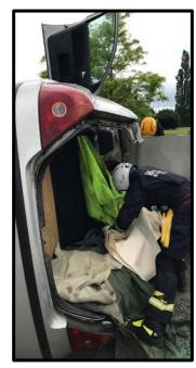
The 'Space Creation' phase should start with an inner and outer structural assessment of the vehicle to determine which components can be moved, opened or manipulated by using the vehicles natural design features. It should also establish what obstructions and hazards will impact on space creating techniques. No tools should be necessary at this stage, you are looking for easy wins and gathering information.
