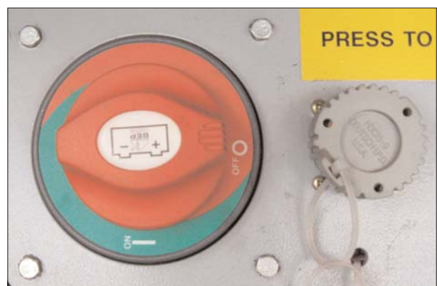
Master Disconnect Switch
