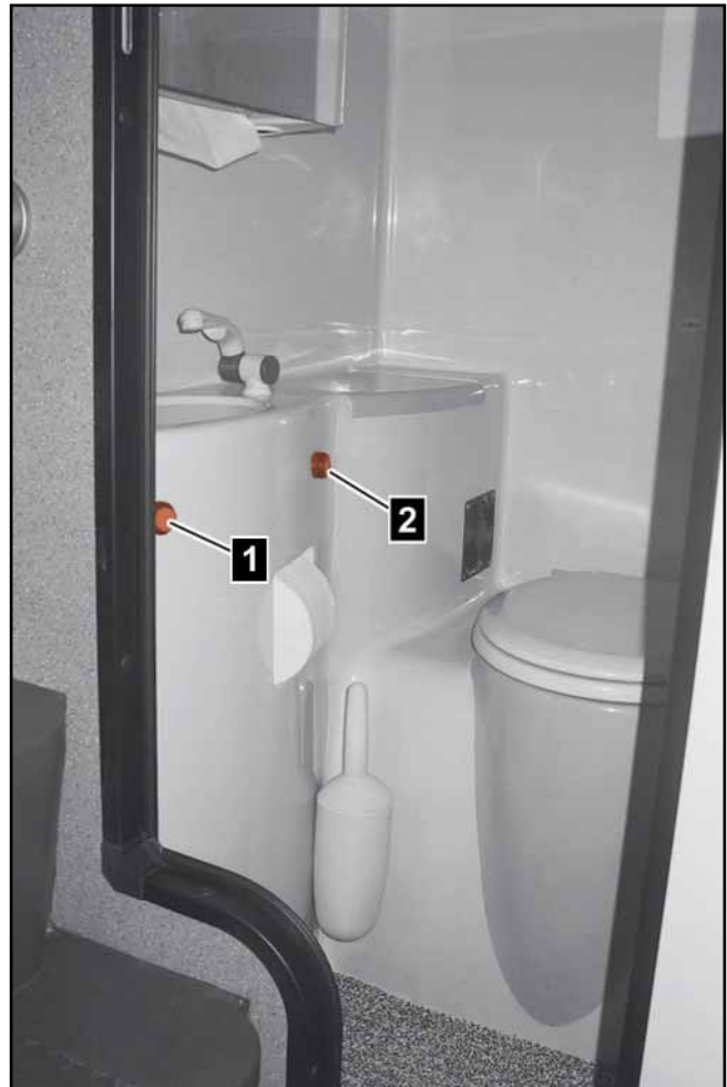
On-board toilet 1 Wash basin water button 2 Toilet flush button
