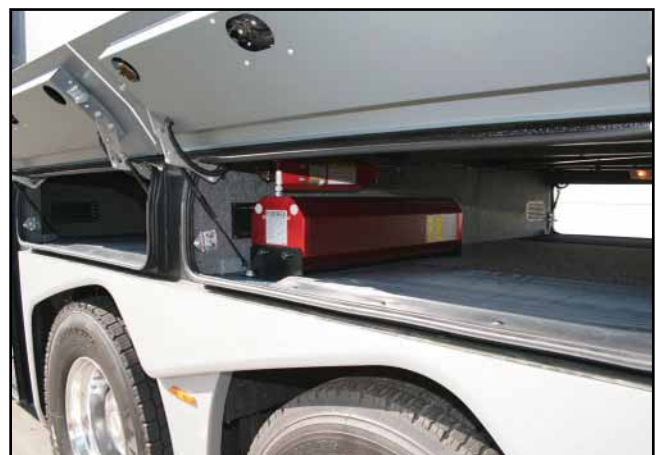
Fire extinguisher tank (example, Starliner)
