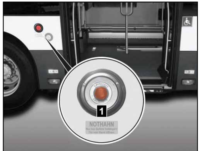
1 Emergency valve outside rear door (example)
