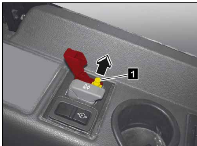
1 EMERGENCY OFF switch (example, NEOPLAN Starliner)
