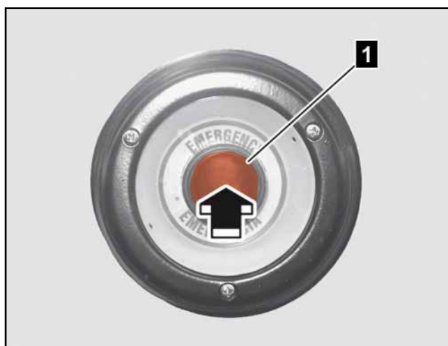
1 Outside emergency valve (example, pushbutton)
