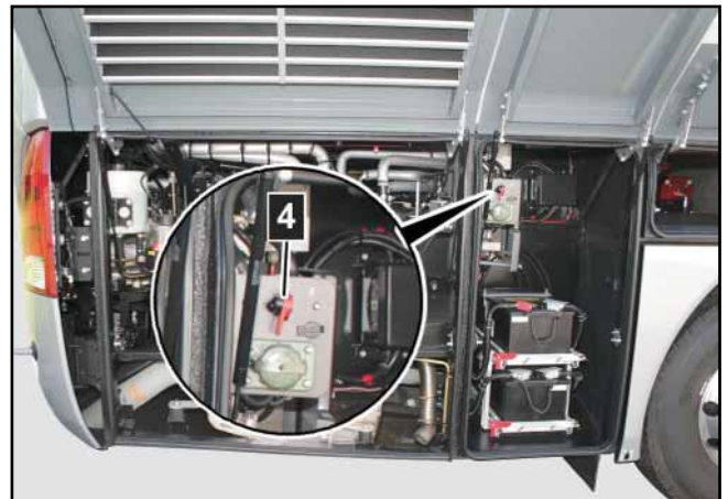
4 Battery isolator switch, coach (example, Starliner)
