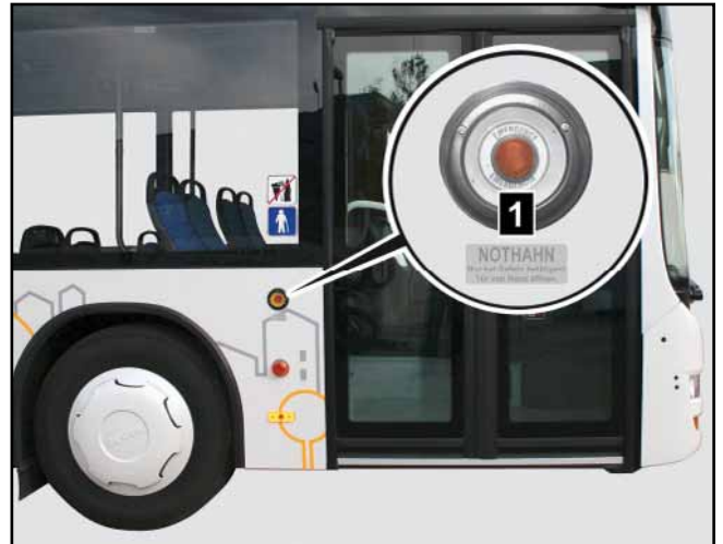
1 Emergency valve outside front door (example)
