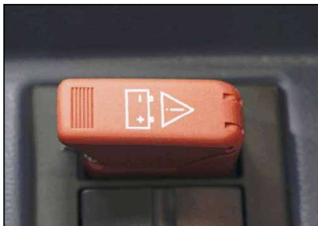
EMERGENCY OFF switch (example, Lion's City Hybrid)
