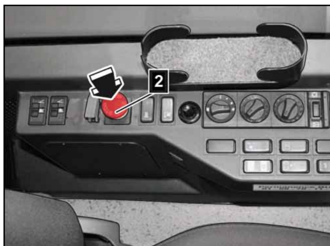
2 EMERGENCY OFF switch (example, Lion's City)
