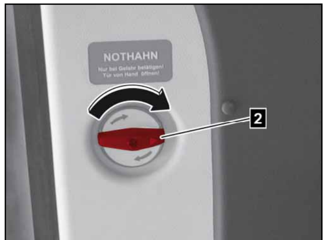
2 Emergency valve, front pivoting door
