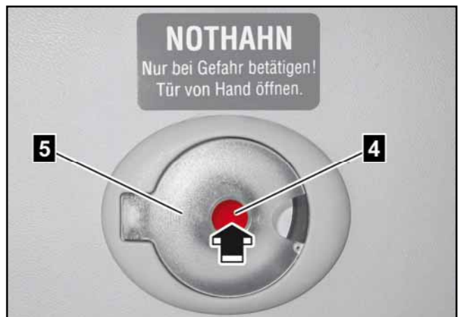
4 Inside emergency valve (example, pushbutton)
