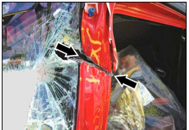
Cut on A-pillar
