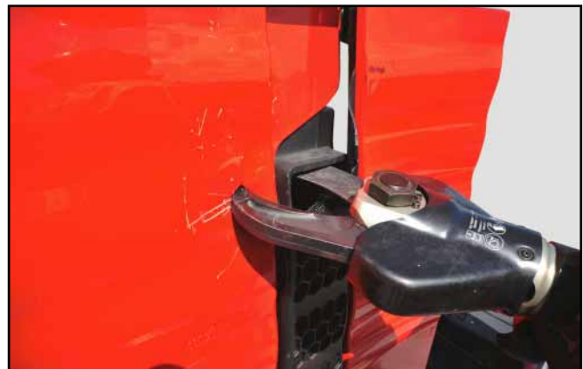
Cut in side wall
