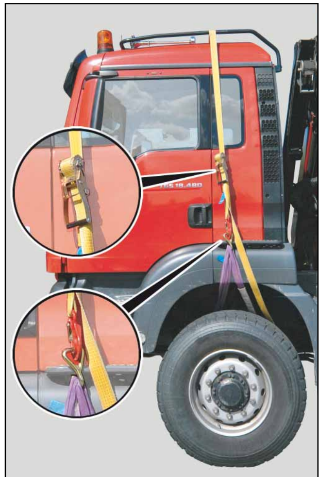
Securing the cab, example shows TGS
