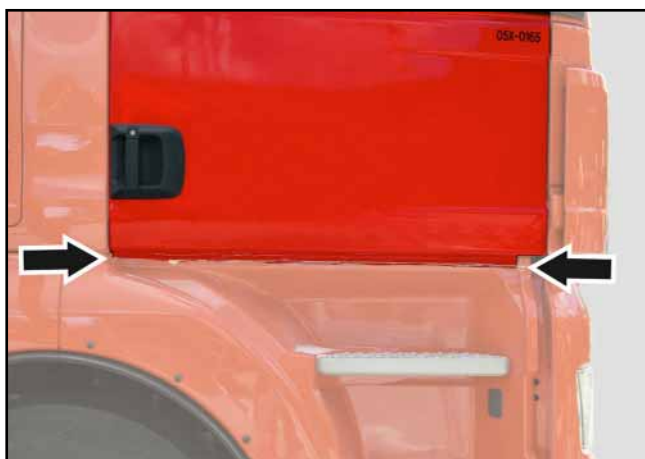
Cut edge of door trim
