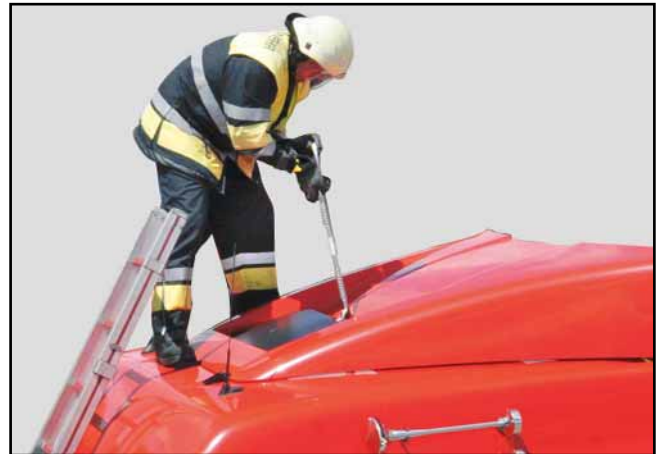
Opening the roof hatch with Halligan bar
