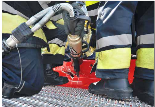
V-cut: Cut in at an angle from the rear
