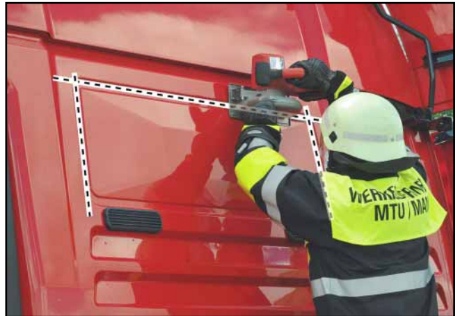
Sawing an opening into the rear wall
