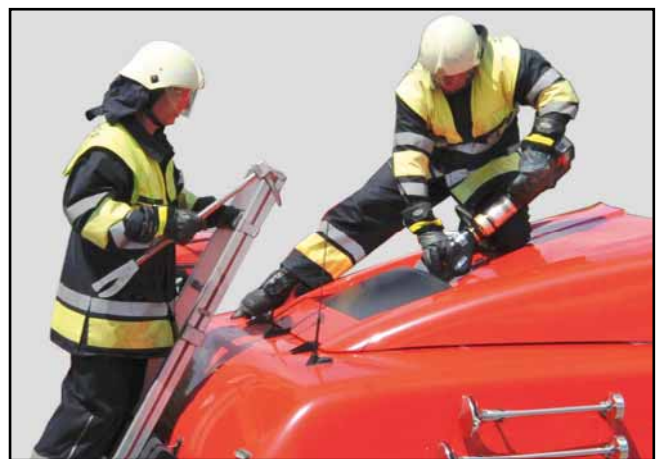
Spreading apart the roof hatch
