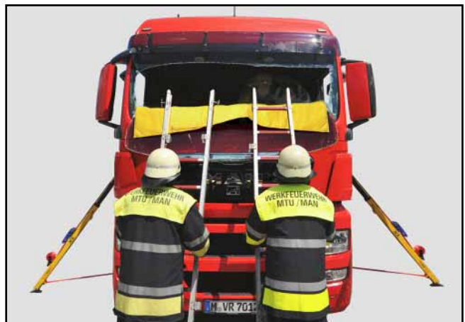
Setting up scaling ladders
