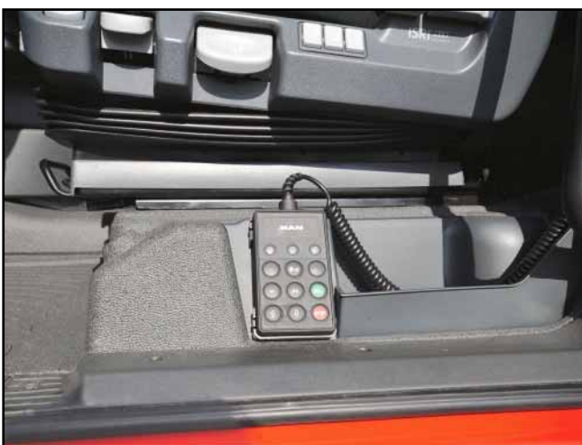
Sample arrangement of control unit
