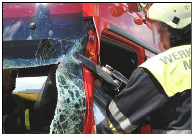
Cut on A-pillar
