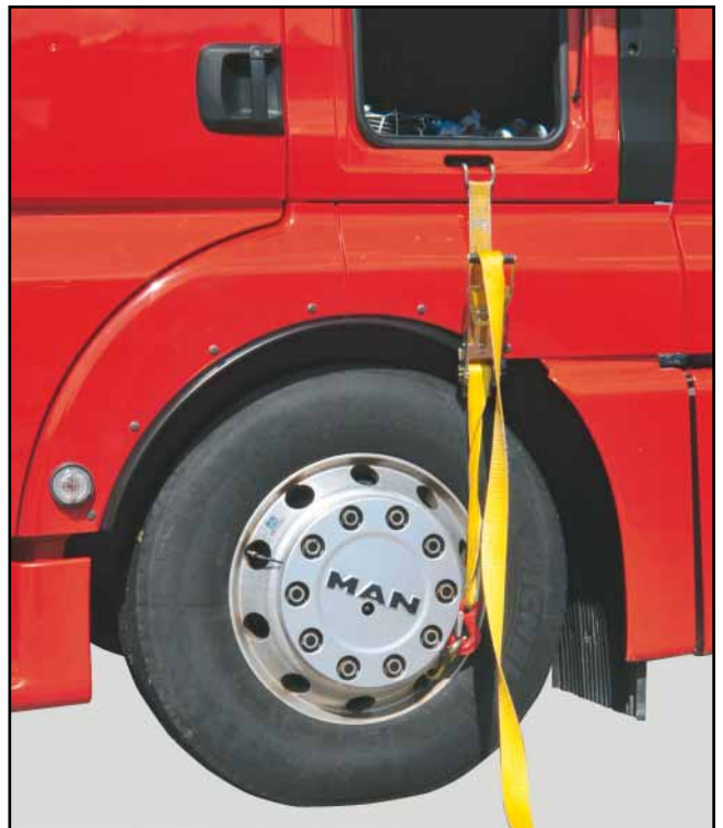
Securing the cab using the storage locker flap, example shows TGX
