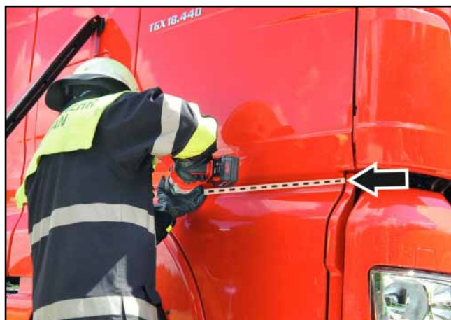
Sawing off the door trim
