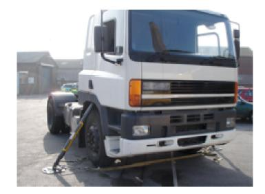
they ensure road shock is minimised in its transmission through the cab and ultimately to the driver. This, for rescuers, means that the cab is an unstable working environment not only for a casualty with a possible cervical injury, but also for the rescuers. For both these reasons its movement needs to be removed or minimised.
