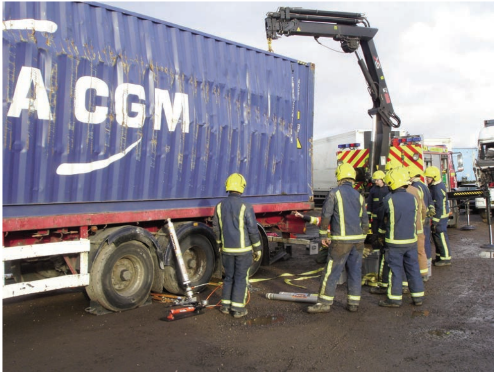
In this picture the rear of the LGV trailer is being lifted by a Lorry Loader Crane and High Pressure Air bags, throughout the process its chassis is being dynamically stabilised utilising vehicle stabilisation equipment and wooden cribbing/ blocks.
