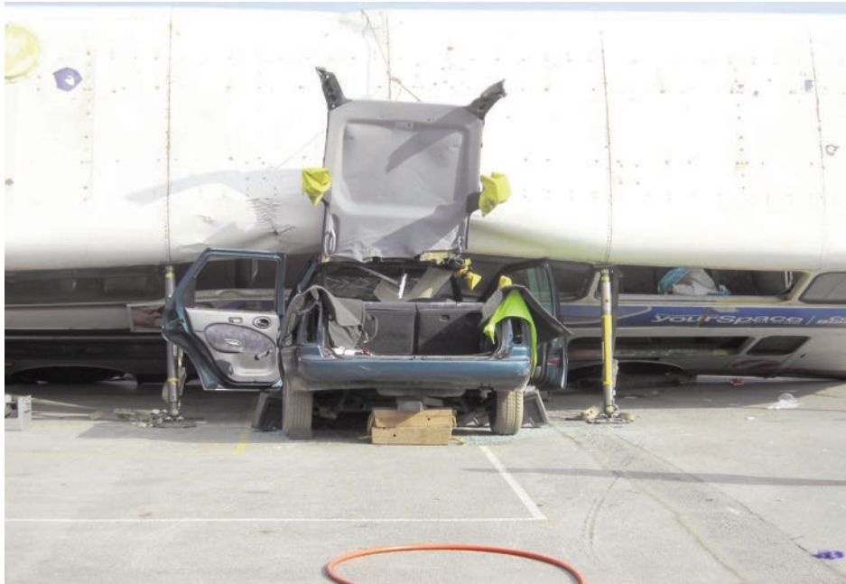
In the above picture employing Static Stabilisation has ensured the PSV cannot move any further and has also provided a "Safety Cell" for the attending Rescuers/ casualties
