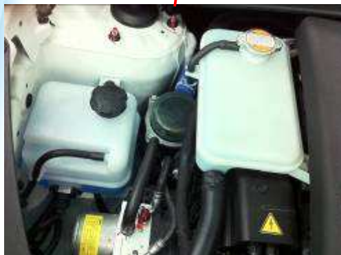
Left: Fuel cell coolant reservoir Right: Electric cooling reservoir
