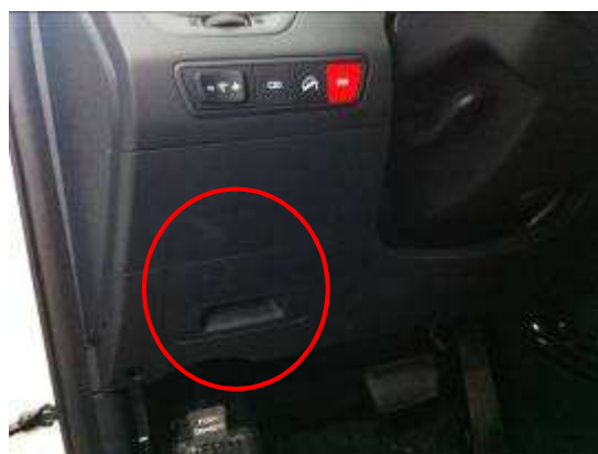
Conventional vehicle system related fuses and relays
