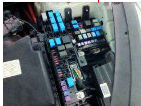
Left: fuse and relay box of fuel cell system Right: fuse and relay box of conventional system
